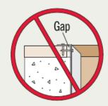
DO NOT install hanger overhanging face of plate or beam. Flush bearing plate with inside face of wall or beam.
