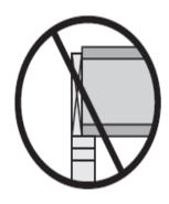
DO NOT use sawn lumber for rim board or blocking as it may shrink after installation. Use only engineered lumber.
